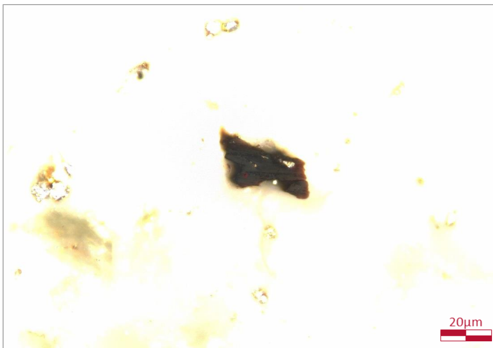
Sample 6126527249 (6908') : Representative vitrinite particle with a reflectance reading of 0.51%Ro from central measuring circle.
