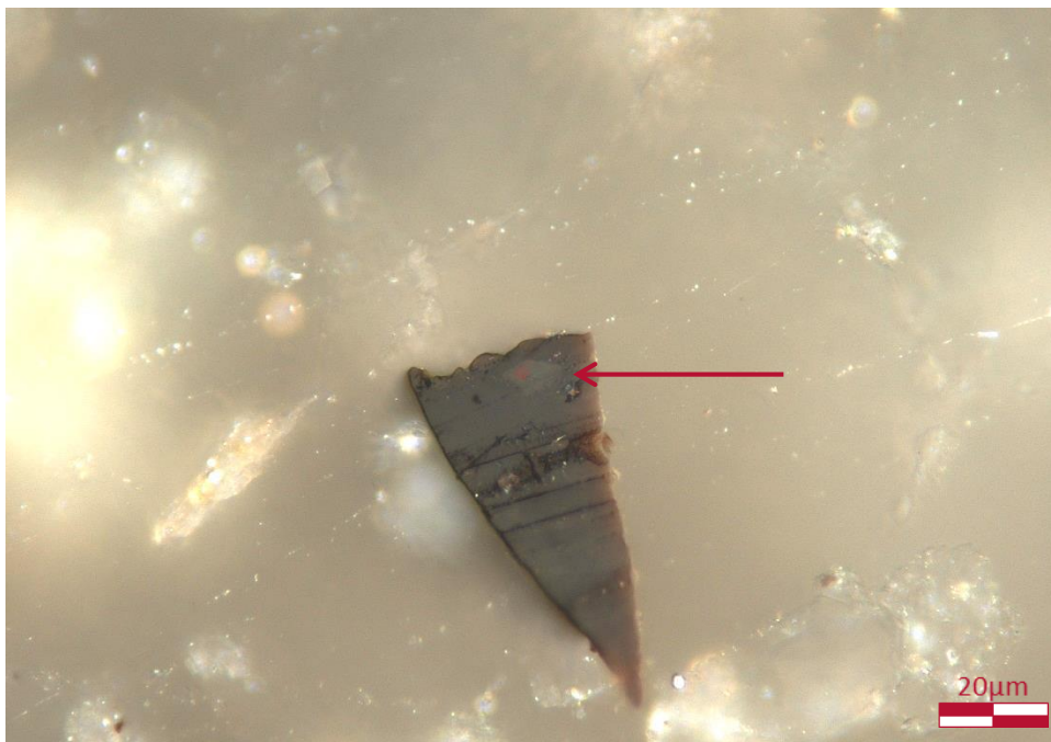
Sample 6126520988 (8280'): Small cell of collotelinite (indicated) with a reflectance reading of 0.58%Ro, within collodetrinite particle with a reflectance of 0.47%Ro.
