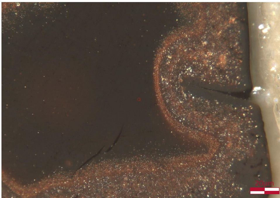
Sample 6126527253 (7705') : Large particle of solid bitumen with desiccation cracks (indicated). Reflectance from central measuring circle is 0.19% Ro.
